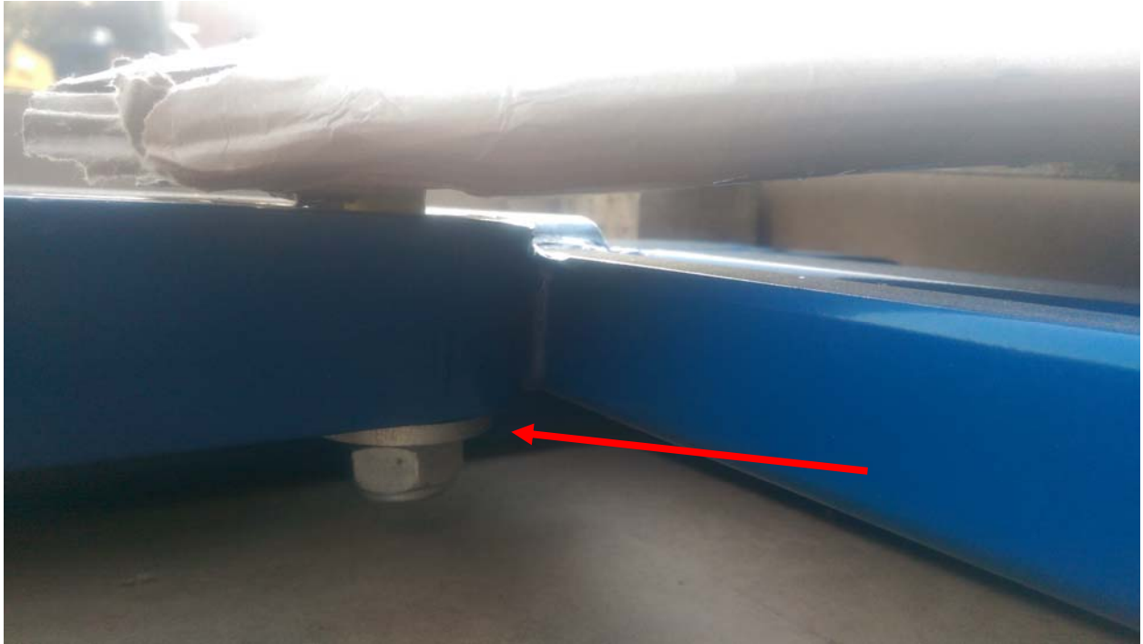
Shown is how the arm will be bolted on to the lift frame with a washer and nut.
