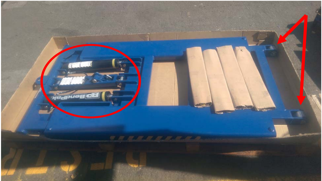
Note: cylinders, all pins, safety assembly, fittings, hose between cylinders and rear rollers are all pre-installed.
